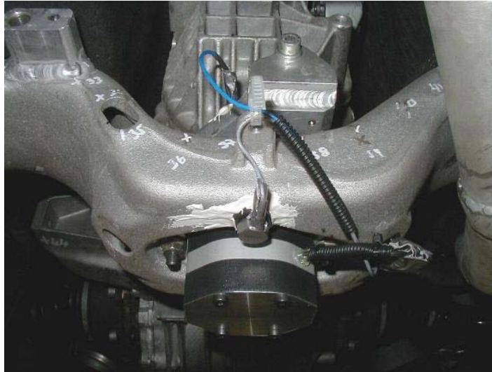
Figure 2: Location of the active absorber and the sensors in a test vehicle.
